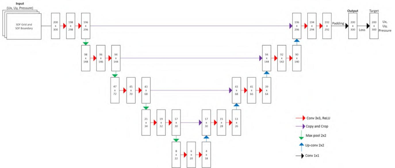
Fig. 4: U-Net architecture for CFD prediction with the contracting path on the left side and expansive path on the right side.
