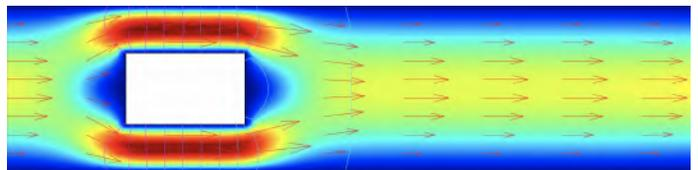
Fig. 1: Sample a non-uniform steady laminar fluid flow for 2D geometry. The white rectangle depicts the obstacle. The pointers indicate the laminar flow's velocity field.
